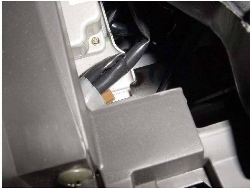
Solder and tape or heat-shrink over the connection
