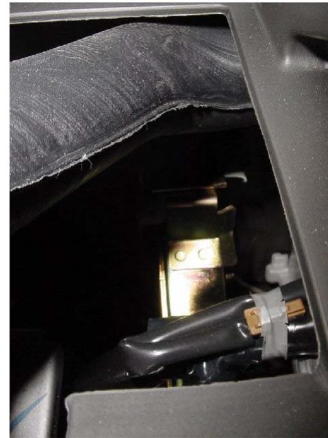
Step 2 - If you look down the hole into the dash, you'll see the factory wiring loom with the tweeter plug and some silver tape holding it in place so it doesn't rattle around under the dash...
