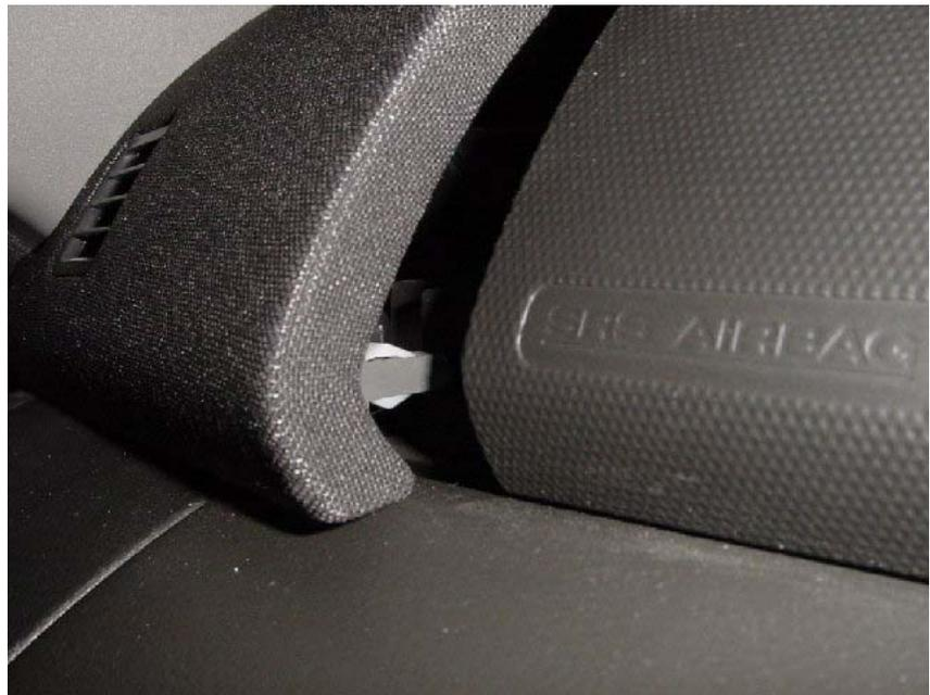
Step 1 - remove grille by pulling towards self and up slightly. Don't panic as the panel is designed to flex abit to be removed easily.
