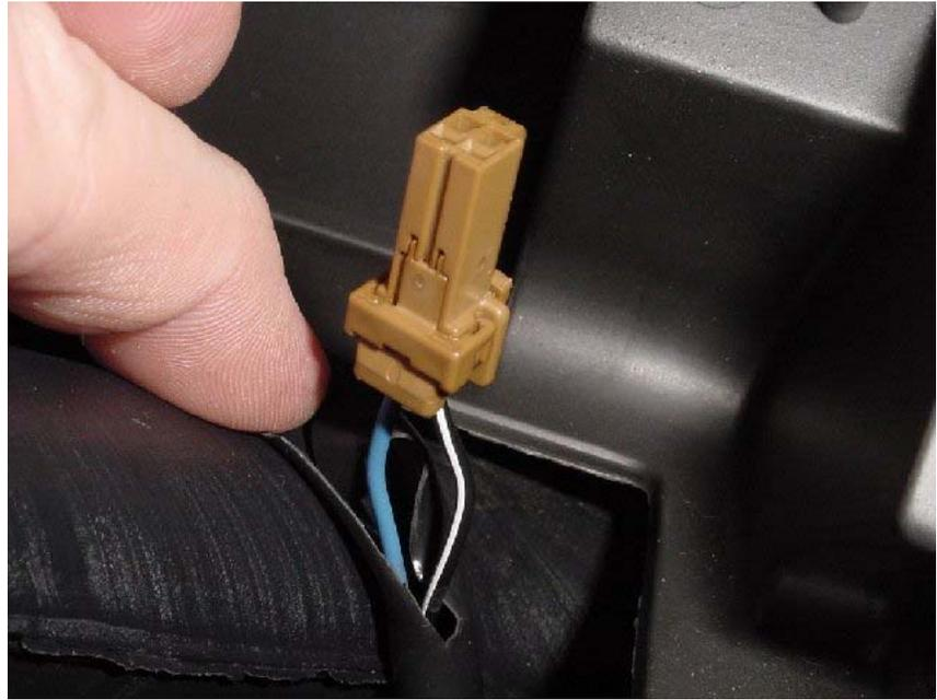
You need to cut to silver tape carefully with a sharp knife so there's abit more cable to play with when you strip the wires. You also need to trim off abit of the black shroud over the two wires so they can be spliced into.
