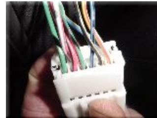
The plug inside the passenger's side "B" pillar which I got ignition "turn-on" and speaker-level inputs for amp
