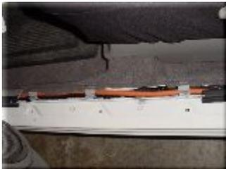
The power cable for the amp running along the sill
