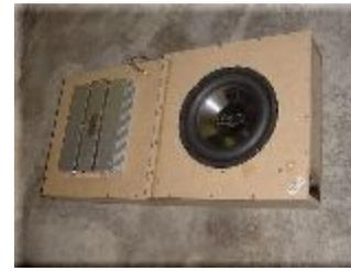
Completed sub box with amplifier and subwoofer mounted
