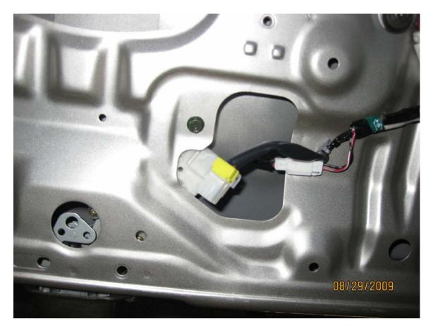
To access the signals, I cut open the heat shrink cover over the wires, and spliced the two wires using a pair of automotive cable splicers for 14-18 gauge wire. These cable splicers have an insulated cover, and I zip-tied both together after the splice to maintain cable integrity. If you are using some other method to splice the wires, ensure that you maintain the cable integrity and insulate the splice appropriately!
