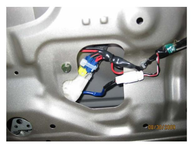
This is the pizeo buzzer I used. To mount this, I first used double sided foam tape to secure the buzzer in place on the underside of the inner frame, then zip tied it in place once everything had been tested. The foam tape also serves as a vibration damper. Note that the wiring has been routed inside the tailgate panel.
