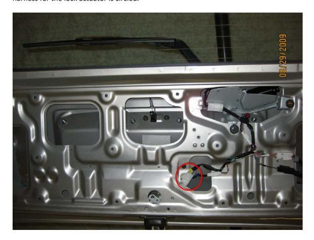
A closeup view of the wriring harness. There are 2 wires inside the connector, a red (R), and a red/green (R/G). In my 2005 XTrail when the lock signal is sent, R is (+), R/G is (-). When an unlock signal is sent, the reverse applies. You should confirm this with a multimeter before proceeding.
