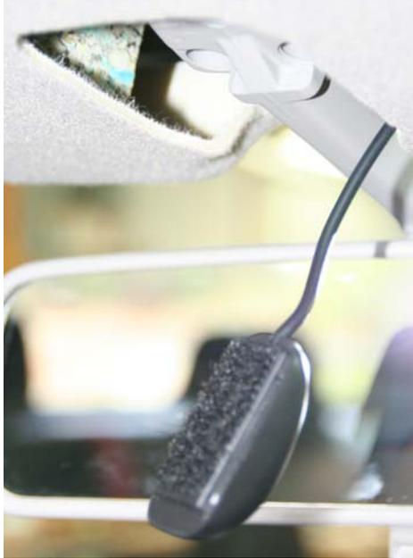
Run the cable through the roof to the door pillar and continue down to the tweeter speaker box.
