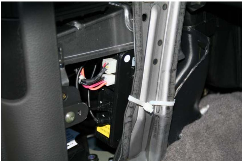
It was secured with two cable ties. The power and speaker harness was easily run down from the stereo harness.
