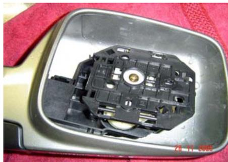
4. You now have access to the internal part of the mirror housing and can pass the wiring through the existing wiring loom. (the easiest way to pass the wires through is to tape them to the existing mirror wiring and pull them through)
