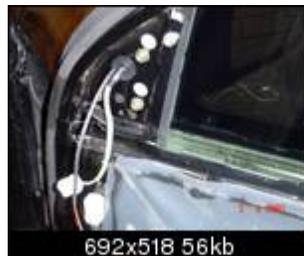
It is now time to take the mirror glass off, so you can pass the wiring through the internal part of the mirror housing:
