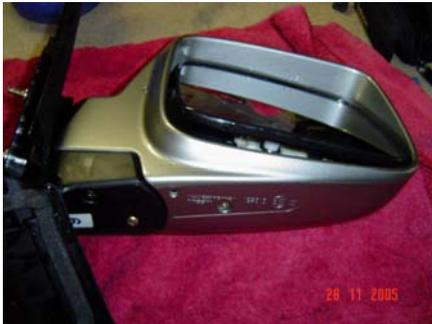
3. Tilt the mirror glass as shown in the above photo and lift the bottom part of it up so it un-clips from its place.
