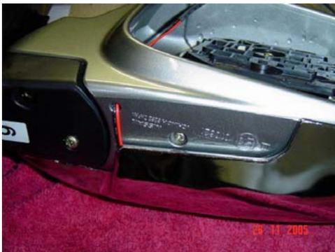
5. You now have the option of using an existing hole in the mirror housing to pass the wire from the LED mirror cover OR drill a hole in the factory mirror housing for a bit better look (making the wire invisible) The choice is yours.
