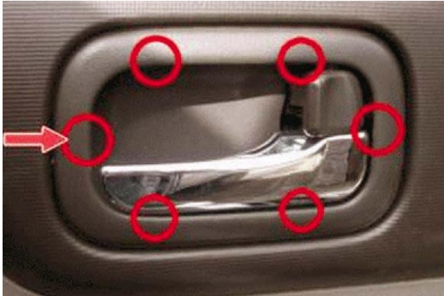
4. You will now be able to unclip the door trim from its place. Start from the edge closer to the door hinge and work your way around the bottom part of the door trim. The red circles show the location of the holding clips.
